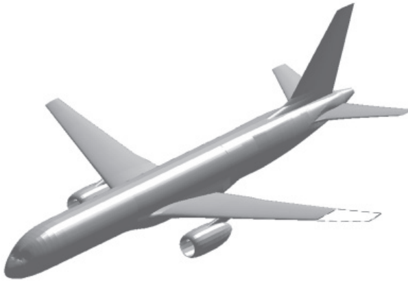
Fig. 2. Left Wing Damaged Generic Transport Model
