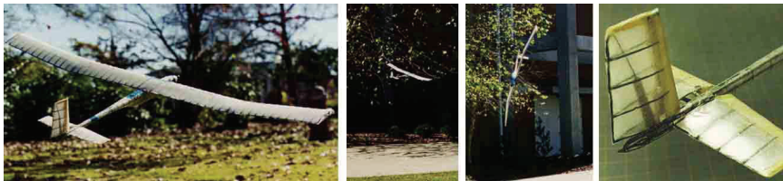
Fig. 13. Mothra , The First UAV with Flexspar Stabilators for Flight Control
